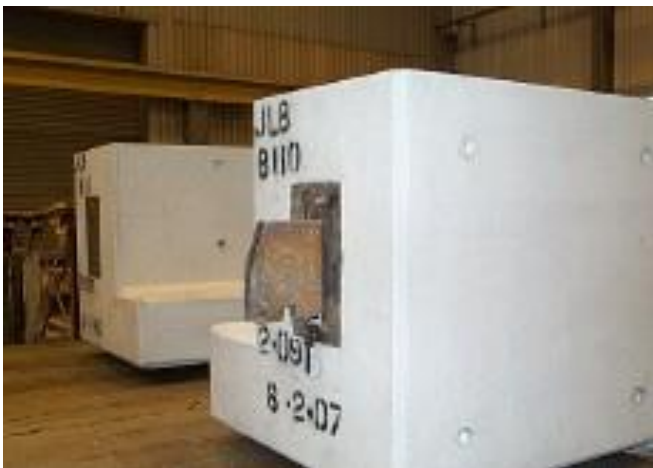
BSF connector in a beam, shown with 'knife' component projecting.
