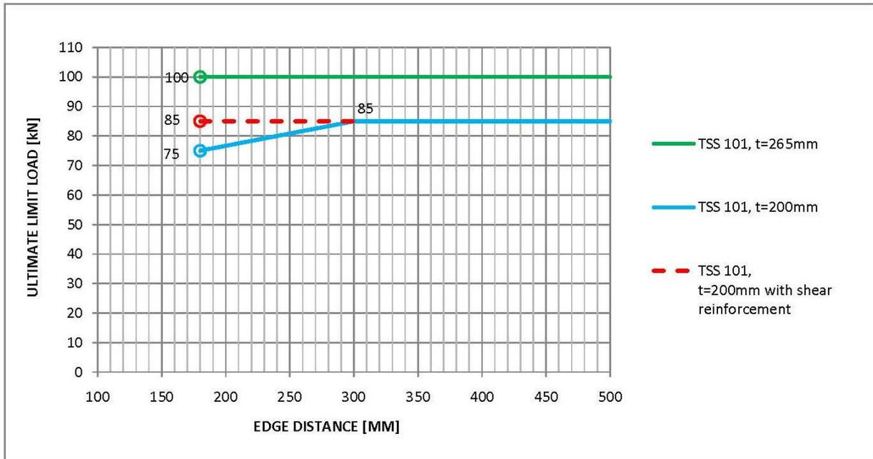
Fig. 4 b. Recommended ULS vertical shear capacity for RVK/TSS 101 in 200-265 mm slabs
