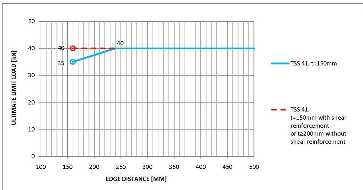
Fig. 4 a. Recommended ULS vertical shear capacity for RVK/TSS 41 in 150 mm thick slab.
