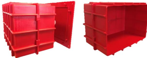
Alternatively, the integral lugs (two on four sides) provide ample fixing points to tie-wire the unit to the wall reinforcement (ideal for slip-forms). The recyclable face-plate incorporates a central 'soft-eye' into which a hammer-claw can be inserted to pull and detach, revealing the clear recess.
