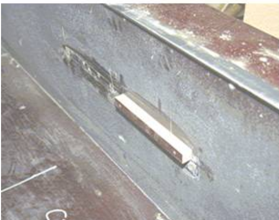
2.5 Guiding knife in right position Important
