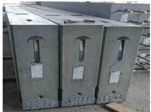
5.6 Finished beams with BSF
