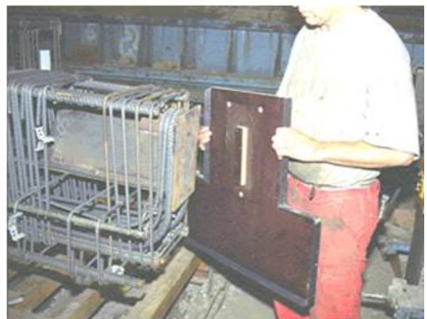
4.4 Endplate with guiding knife Important
