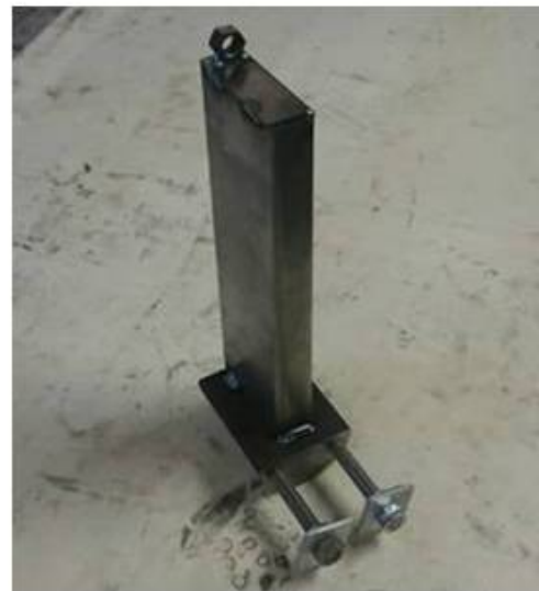
3.4 BB unit with threaded bars and washer
