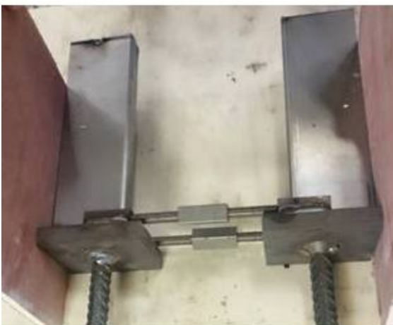
2.3 Shorter bars connected with thread sleeve
