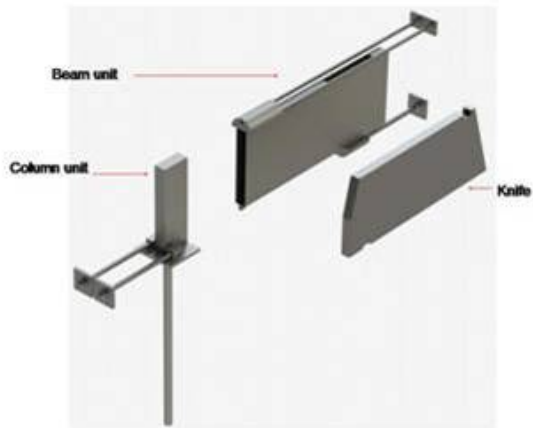
1.1 BSF- , column unit, beam unit and knife
