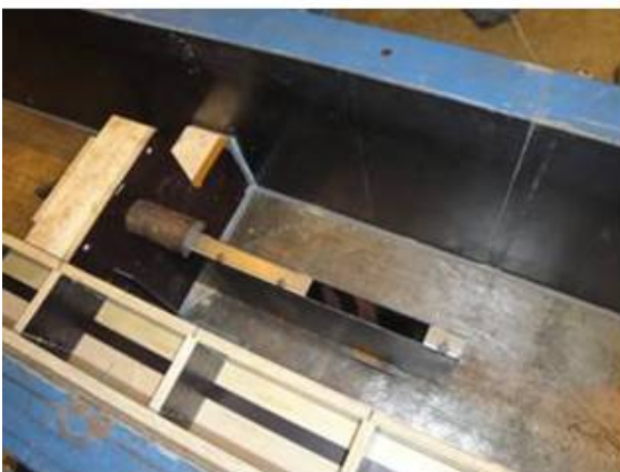
4.5 Endplate with guiding knife Important
